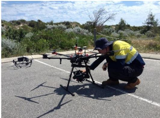
The camera used to capture the images – a SONY A7RII 42MP - provided an image resolution of 1 cm (on the ground) per pixel.
